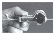
2. Determine desired degree of tension and dial to proper setting.
